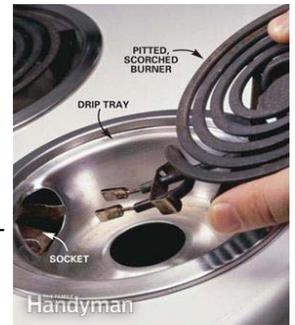
If the **issue is with all burners**, there is probably a larger issue. If your stove has a built-in digital clock/timer but it is not displaying, or if it is part of an oven and the oven light won't go on, you probably don't have any power to the unit. Please see the section on Circuit breakers. If the problem persists, this is not an emergency, contact the office to schedule a service repair.
